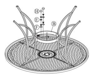
Step 4: After making any necessary adjustments to the alignment of the table legs and the leg connector bracket, use the hex bolt driver and hex wrench to tighten all nuts and bolts. Note: each bolt and nut must be tightened a few revolutions at a time. In order to apply equal pressure to all bolt joints, we recommend working in a cross corner (X fashion). Repeat until all bolts are tight. Do not over tighten. Over tightening may strip bolts. Cover all nuts and bolts with covers.
